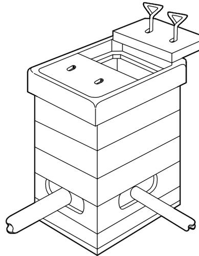
Minimum Cross Sectional Area of Chamber 0.25m<sup>2</sup> up to 1000mm deep
